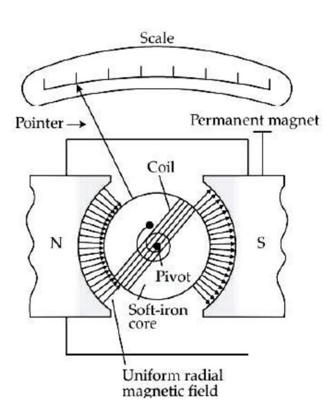
In moving coil galvanometer, current in the coil will be directly proportional to the angle of the deflection of the coil,  $I \propto \theta$
